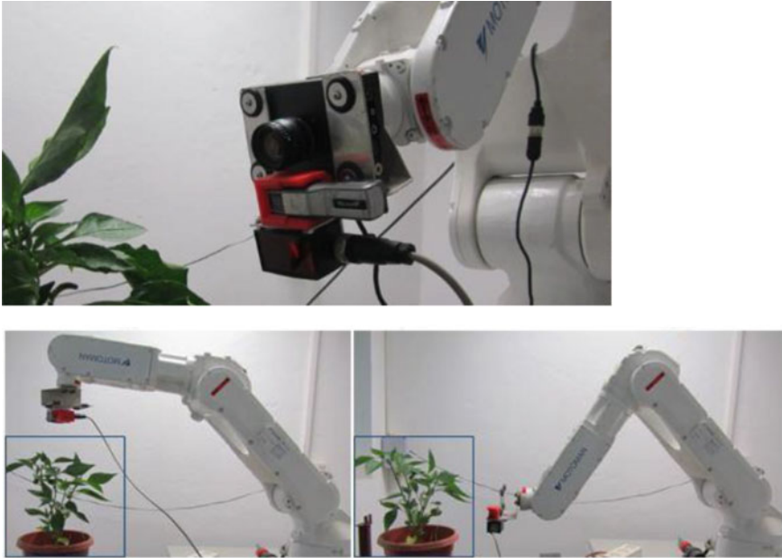
Fig. 8.15 The apparatus for disease detection for pepper plants (Source Agricultural Research Organization, Israel)
