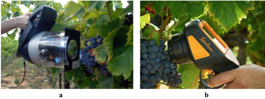
Fig. 5.3 Handheld maturity assessment: a Spectron® (Pellenc) and b Multiplex® (Force-A)
