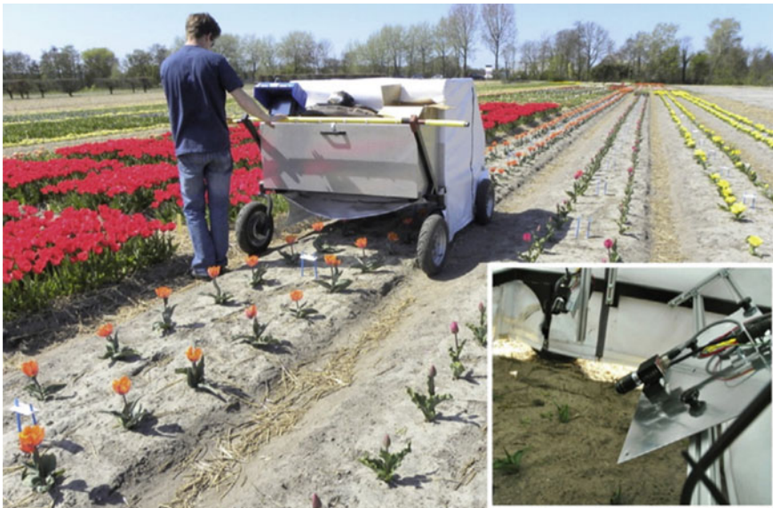
Fig. 6.4 Sensing platform for detecting tulip breaking virus (TBV) disease. The right inset shows the interior of the fully enclosed imaging area for obtaining controlled illumination ( source Polder et al. 2014)
