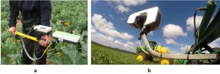
Fig. 5.2 Ground-based NDVI estimation: a CropCircle ® ACS-470 kit as a handheld device and b GreenSeeker ® RT200C mounted on a conventional farm vehicle
