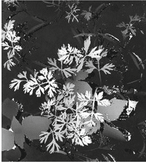
Fig. 6.1 Depth image of carrot plants and weeds: brighter pixels (the taller carrot leaves) are closer to the top-viewing camera than the darker pixels (lower weeds foliage). The image shows the great potential of 3D approaches in crop–weed discrimination ( source Piron et al. 2011)
