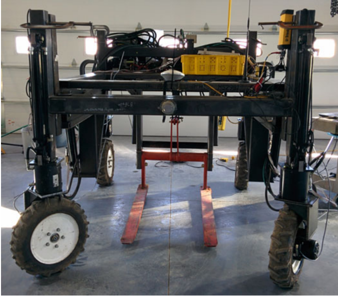
Fig. 4.11 An automated bin handling machine (also called automated 'Bin Dog') developed at Washington State University
