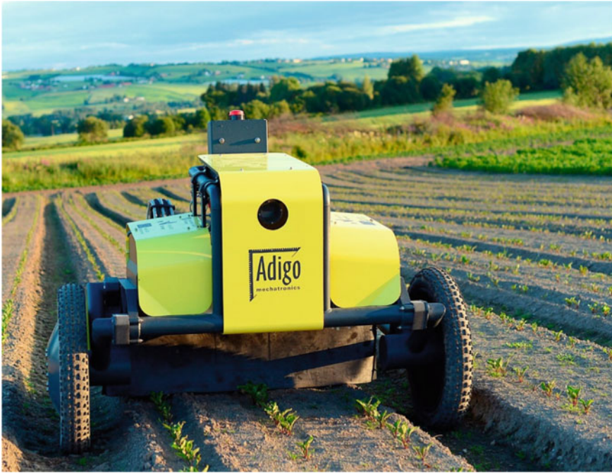
Fig. 6.8 The weeding robot Asterix is an example of ultra-precision spraying robot. The individually controlled micro-spraying nozzles can apply herbicide selectively on sub-centimetre weed seedling targets ( source Utstumo et al. 2018)
