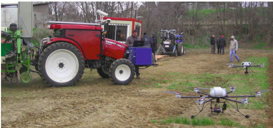
Fig. 6.7 The cooperative fleet of robots RHEA. The UAV platforms (on the right) have the task of remote monitoring of fields for weed detection; the processed data are sent to autonomous ground platforms (on the left) for physical weeding or selective spraying of herbicides (source Gonzalez-de-Santos et al. 2017)
