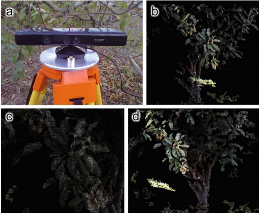
Fig. 3.4 Microsoft Kinect version 1, a low-cost consumer grade depth camera (structured light sensor and RGB camera) with potential applications in agriculture (a) and different views and details of 3-D point cloud with RGB data for each pixel of a medlar tree ( Mespilus germanica L.) captured by the Kinect v1 depth camera (b, c and d)
