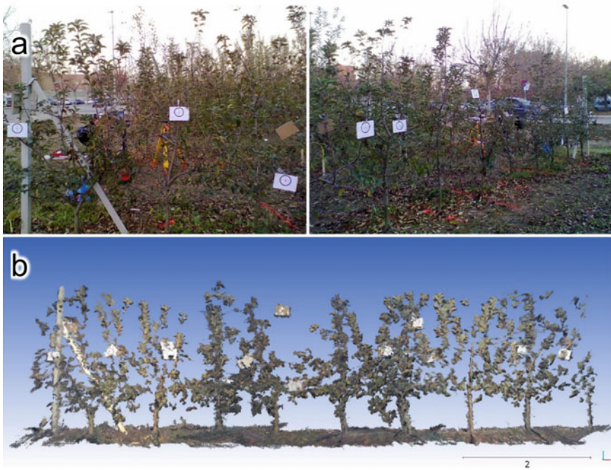
Fig. 3.14 Row sections of an apple orchard (a) and point cloud obtained with a Microsoft Kinect version 1 sensor (b)
