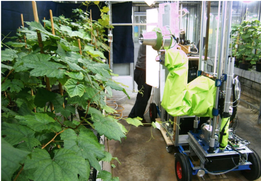
Fig. 6.9 The multifunction agricultural robot CROPS equipped with a precision-spraying end-effector during an experiment of selective treatments on powdery mildew disease in grapevine. This is among the first examples of fully autonomous disease treatment, with selective spraying targeted on symptoms detected by an on-board sensing system (source Oberti et al. 2016)
