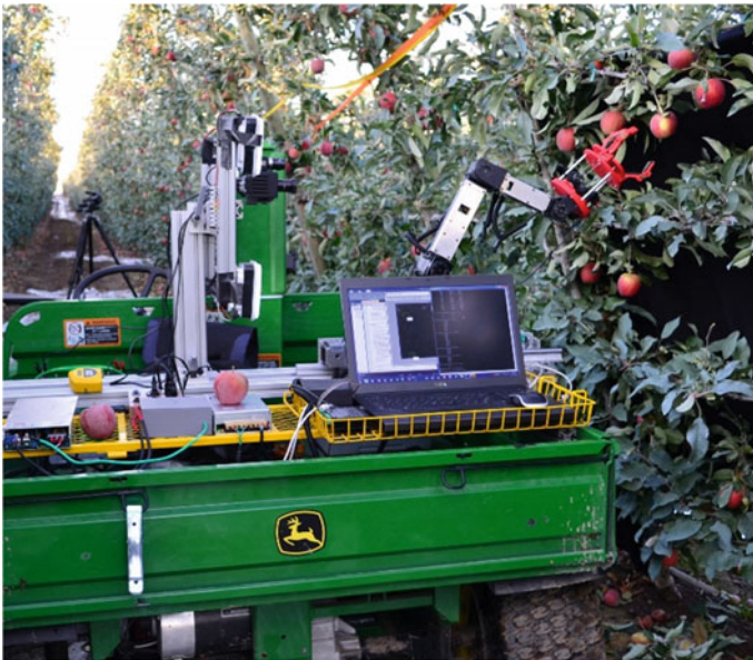
Fig. 4.10 A prototype robotic apple harvesting machine developed at Washington State University is being evaluated in a commercial fruiting wall orchard (Prosser, Washington, USA)
