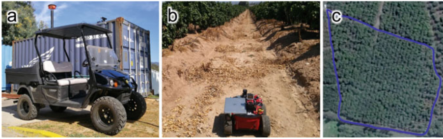
Fig. 3.8 Service units in agricultural environments: an all-terrain vehicle used for agricultural purposes in Chile (a); a Pioneer 3AT robot (b) specially equipped for scouting in an avocado grove in Chile (c)
