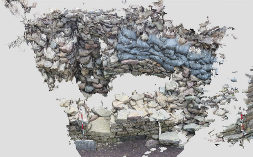
Fig. 14.6 Dense point cloud of Structure 9 northern cell and outer wall, produced in Agisoft Photoscan Professional Edition, from digital images taken in 2015, saved as JPEGs. Note how the outer wall (foreground) has a distinct wave pattern of distortion. The red and white scale bar (centre left) is 1 m in total height (L. Sou)
