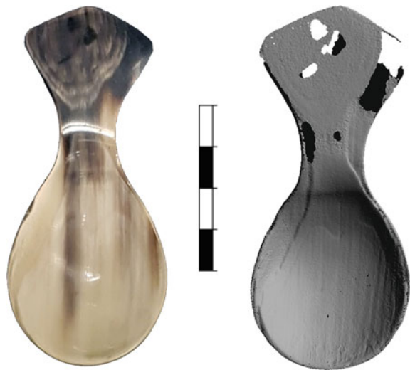
Fig. 10.10 A highly polished horn spoon (left) with its 3D scan (right) showing the problems caused by specular reflection and variations in colour and translucency. (After Holland 2017, pg 117)
