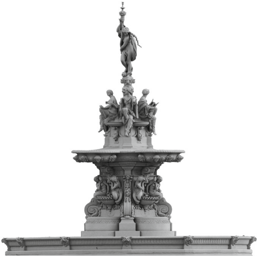
Fig. 16.14 Orthographic render of Ross fountain, visualised with an ‘ambient occlusion’ map to show the geometric data captured by digital documentation
