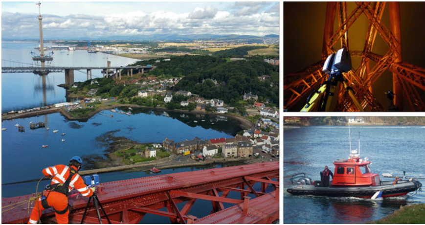
Fig. 16.16 Photo montage of laser scanning the Forth Bridge
