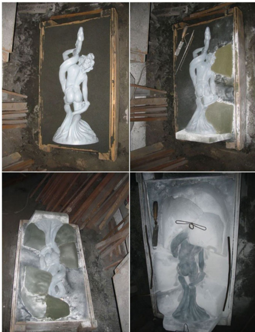
Fig. 16.10 CNC milled and finished model being used to create a loose pattern sand mould
