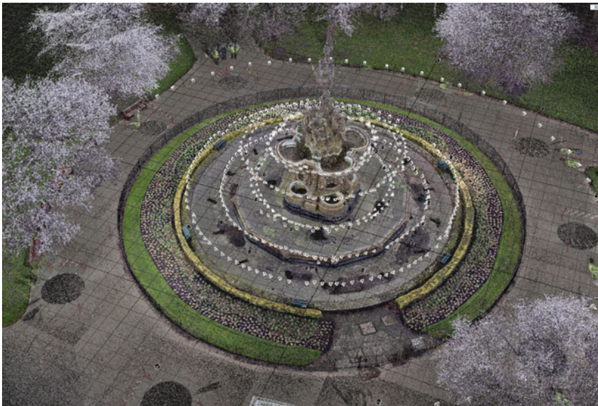
Fig. 16.13 Alignment of 3D laser scans and DSLR photographs in Reality Capture software
