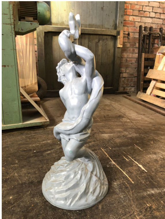
Fig. 16.9 Final CNC milled figure which has had details corrected and has been sealed
