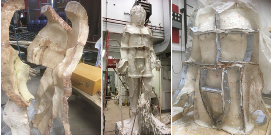
Fig. 19.6 Mould development. Mould torso front and back sections ( left ) first published in Johnson (2020); fabrication of the piece mould approaching completion ( centre first published in Johnson (2020)—both images reproduced with permission from the organisers of the 6th International Conference on Visual Culture); mould flange reinforcements after first casting attempt failure ( right ) (Smartphone photos by Kate Johnson)
