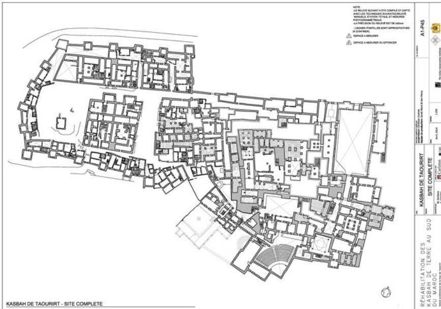
Fig. 3.9 Line drawing for the rehabilitation plan of the Kasbah of Taourirt (Prepared for The Getty Conservation Institute using various recording methods)
