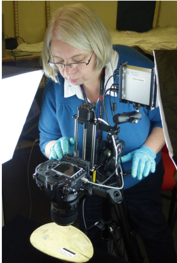
Fig. 10.4 Equipment for focus-stacking photography. Details in text (S.O'Connor)
