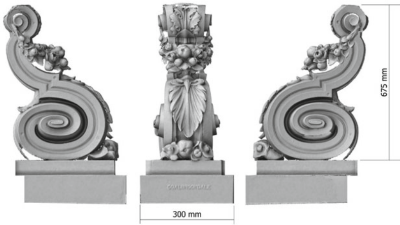
Fig. 16.7 Foot detail scanned with an Artec MHT structured light scanner
