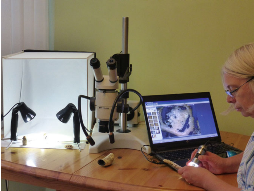
Fig. 10.2 Low cost, portable equipment for the visual identification of animal hard tissues including a Wild Heerbrugg M8 stereomicroscope, a Meiji Techno FT190/240 fibre optic lamp, a Panasonic Lumix DMC TZ6 16 megapixel compact camera, a small folding photographic booth with two table-top LED lights; and a Dino-Lite AM-7013MZT, 5 megapixel digital microscope with polariser (S. O'Connor)
