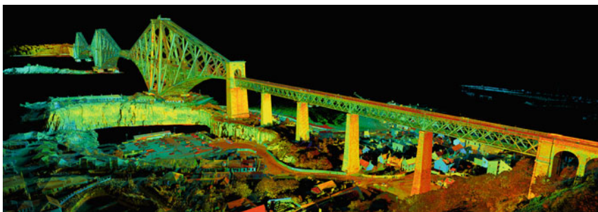
Fig. 16.17 Registered georeferenced point cloud of the Forth Bridge
