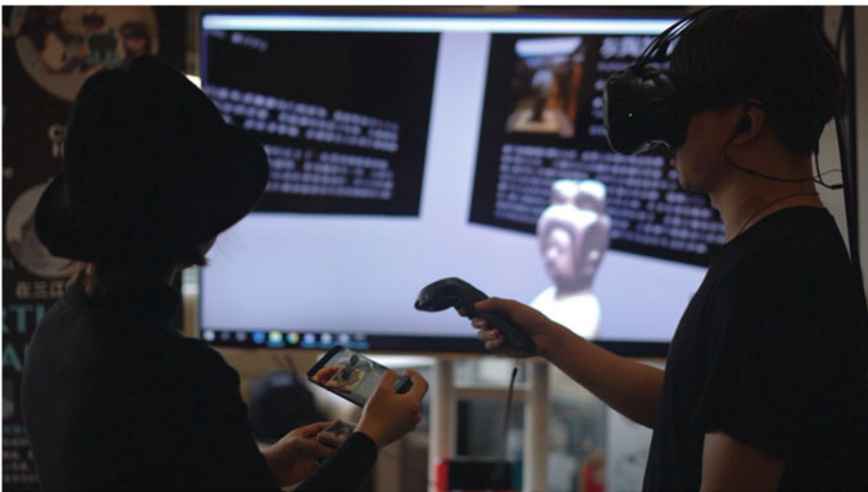
Fig. 23.9 Paired users looking at a shared virtual object in HVAR, one in VR using the HTC Vive (right), and the other with the smartphone AR application in combination with the AR cube (Y. Li and E. Ch'ng)
