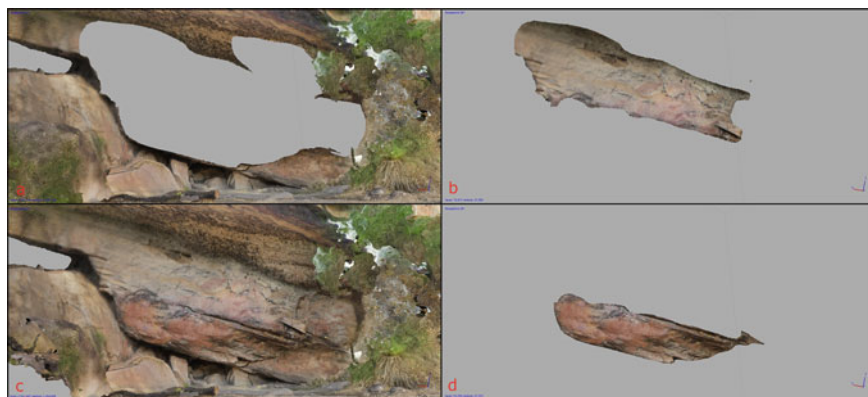
Fig. 6.4 Original model with panels individually extracted (a), individual panels (b, d), the final model with separately textured panels merged back into one mesh (c)
