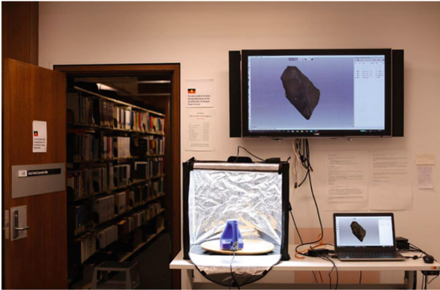
Fig. 5.2 Artefact Conservation Atelier is a smaller Lab containing a 3D scanner, reflective 3D scanning light box (2019), University of Newcastle (Australia). Courtesy UON
