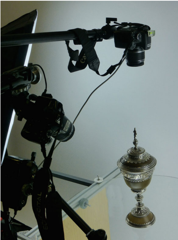
Fig. 10.8 Equipment and set-up for taking an object movie. Object: Leeds Museums (S.O'Connor)
