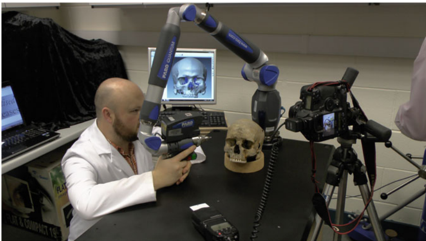
Fig. 22.2. 3D capture of the Winterbourne Stoke Cranium using the FARO Quantum Arm with V3 laser (A. Wilson)
