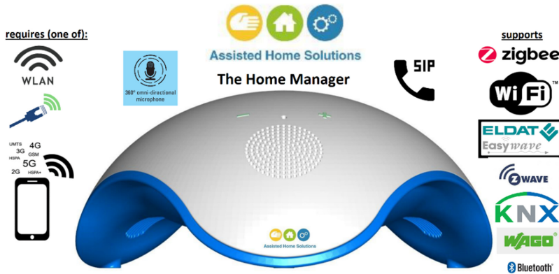
Fig. 3. The first controller with uLive as operating system and the set of supported protocols for binding off-the-shelf components
