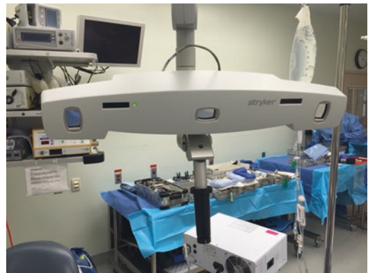
Fig. 13.3 Optical Tracking System that can be moved around to improve “line of sight”
