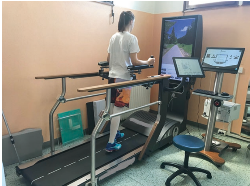
Fig. 23.2 Treadmills equipped with digital mirror able to detect every single angular movement of the runner
