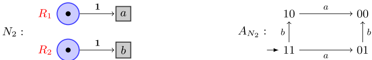
Fig. 3. Left: The Petri Net N_2 with initial marking M_0(R_1)M_0(R_2) = 11 and (0, 1) -restricted places. Right: The reachability graph A_{N_2} .
