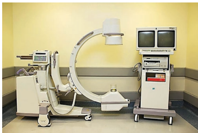
Fig. 14.2 Portable C-arm for fluoroscopy with accompanying mobile imaging screens and recording apparatus
