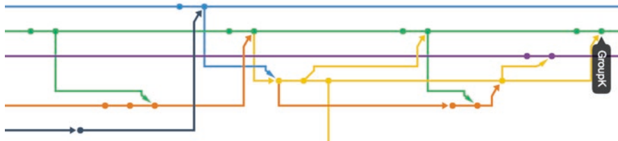
Fig. 7.3 The version history graph shows when different branches of development diverged and merged. Typically, in a software development toolchain, many of the merges into the master branch will have been automatically tested and analysed, providing snapshots of the quality of the code at points in time
