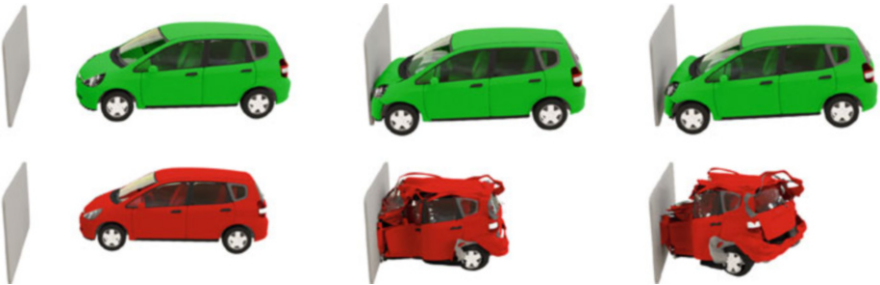
Fig. 3 Simulations of two frontal nonelastic crash scenarios: a car with moderate velocity (top) and high velocity (bottom)
