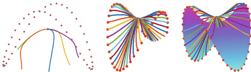
Fig. 3 Surface generation with integral-based Laplace coordinates. Left: several trajectories of proposed anti-gradient flow -\nabla_{\mathbf{x}}A(\mathbf{x}) converge to a single stationary point. Middle: A surface patch is generated by the trajectories of -\nabla_{\mathbf{x}}A(\mathbf{x}) emitted from the boundary vertices. Right: the minimal surface spanned the boundary curve is added; its shape is similar to that of the surface generated by the trajectories
