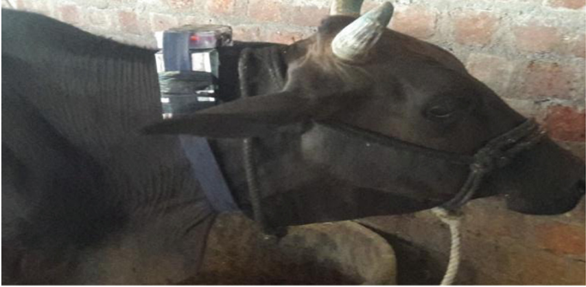
Fig. 4. Positioning of wearable device on the cow's neck
