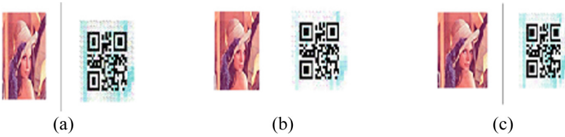
Fig. 4. (a) Gaussian noise (b) Salt and pepper noise (c) Speckle noise
