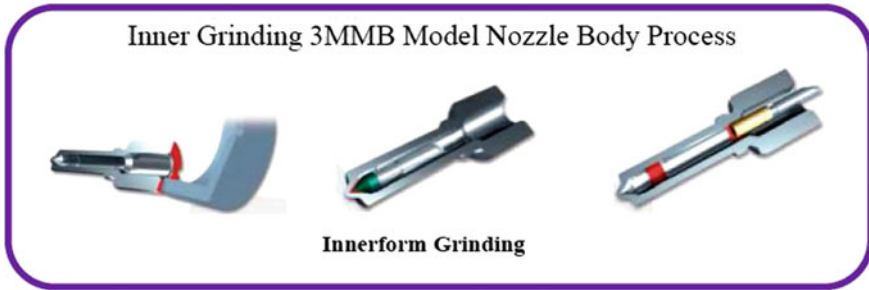
Fig. 5 Inner grinding 3MMB model nozzle body process [8]
