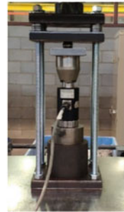
(f) Loading frame developed in Magnel-Vandepitte Laboratory
