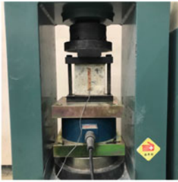
(a) Loading frame for applying compressive load [9]
