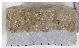
Fig. 3 Colorimetric analysis with AgNO 3 on specimen of OPC and FA mix after chloride migration testing according to NT BUILD 492
