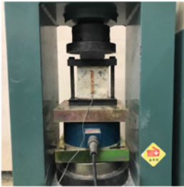
(a) Loading frame for applying compressive load [9]
