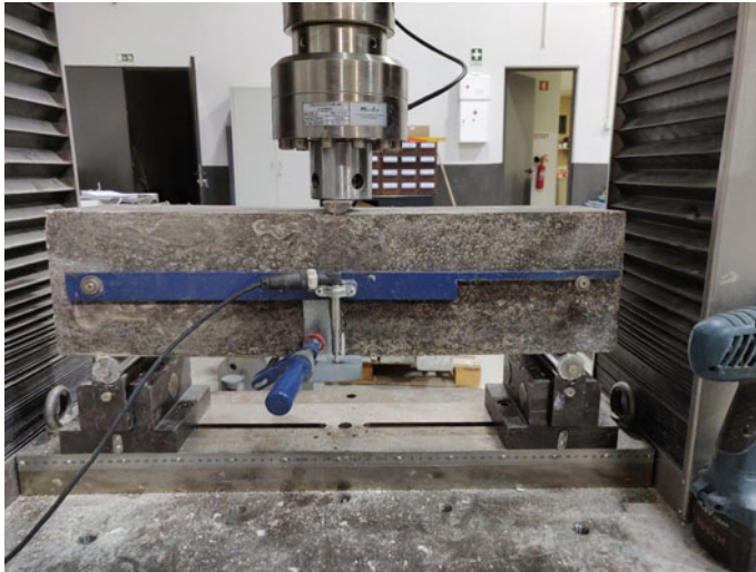
Fig. 2 Setup of the 3-point bending tests
