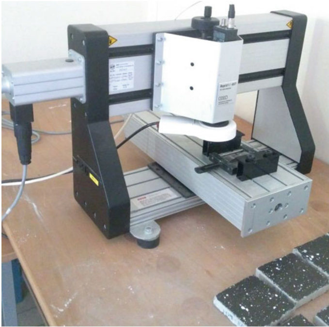
Fig. 3 RapidAir used to perform air void distribution analysis
