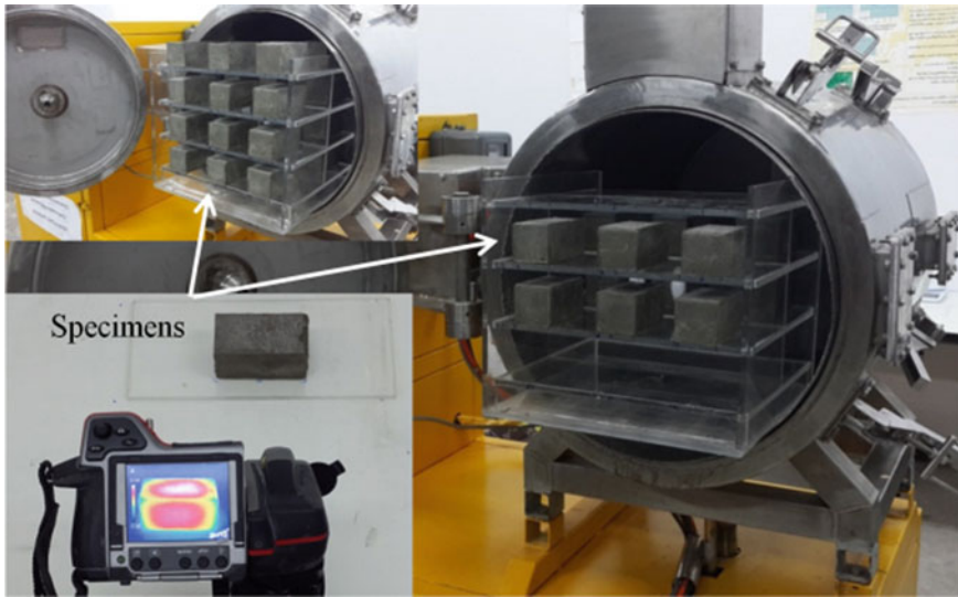
Fig. 1 HSPC specimens after applying the low-pressure MW curing
