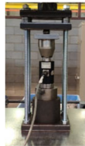
(f) Loading frame developed in Magnel-Vandepitte Laboratory
