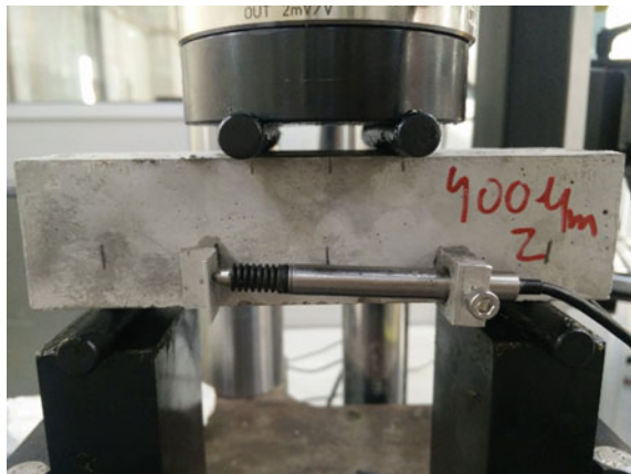
Fig. 1 Four-point bending test cracking method
