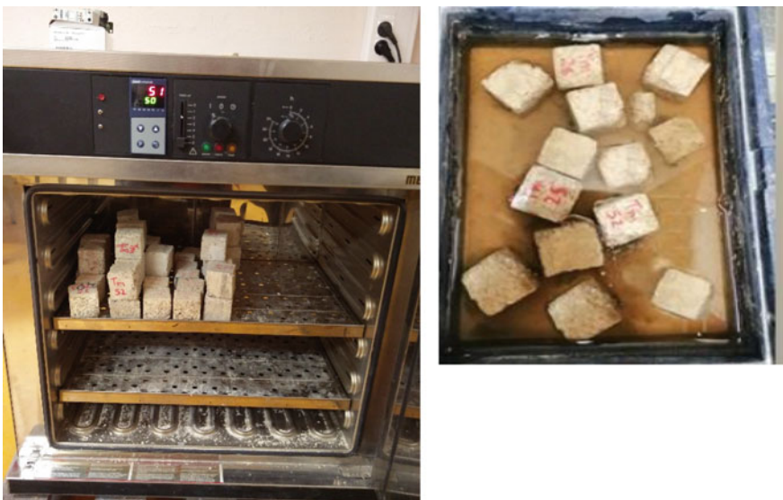
Fig. 2 Hemp concrete sample conditioned in the oven for drying (left) and immersed in water (right)
