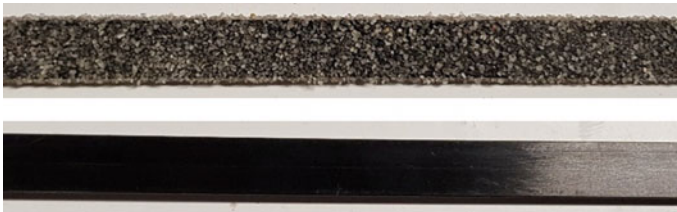
Fig. 1 Sand treated (top) and smooth (bottom) surface CFRP laminates
