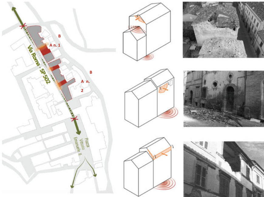
Fig. 3 Critical urban context: the damage state of three structural units of building aggregates
