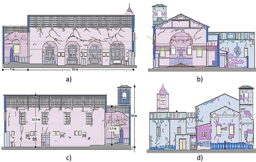
Fig. 3 Damage state of the church: a, b longitudinal section along the nave; c transversal section in the nave; d transversal section passing through the sacristy; e rear view of the church
