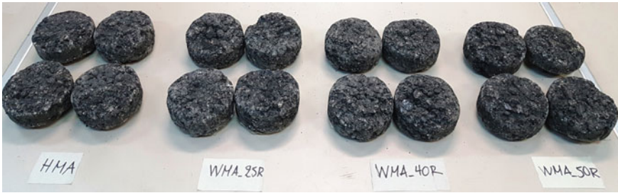
Fig. 4 Specimens of HMA and WMA-RA mixtures after Cantabro tests
