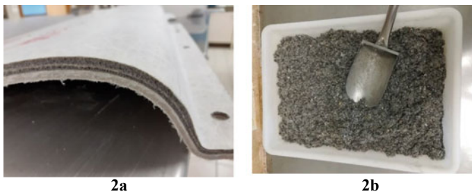
Fig. 2 Waste before (a) and after (b) the grinding
