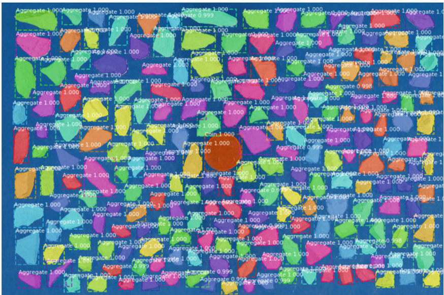
Fig. 7 Bounding boxes and masks extracted using mask R-CNN. Note that the colours of the masks do not represent the sub-class of the grains. They are just used to differentiate different grains
