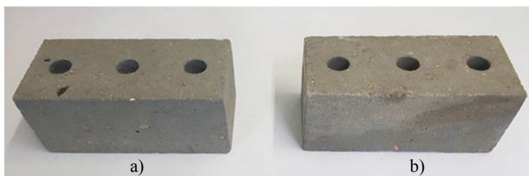
Fig. 6 CWBs with different percentage of PU waste: a PU2.5, b PU5
