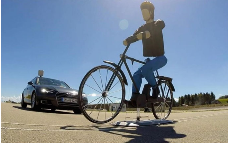
Fig. 9 Autonomous Emergency Braking tests for vulnerable road users were first introduced in 2016 for pedestrians and in 2018 for cyclists
