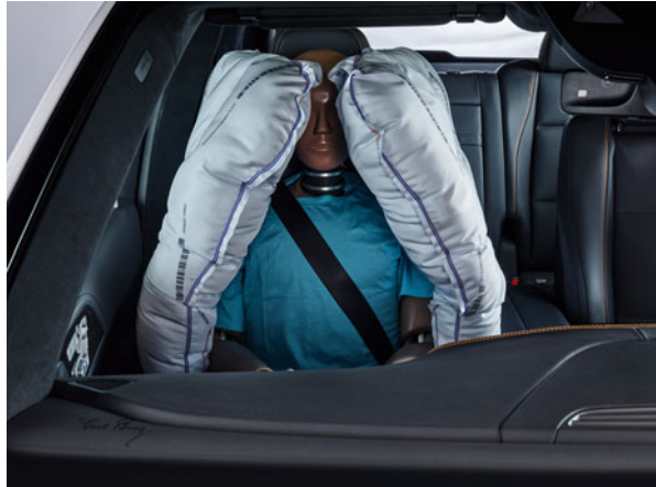
Fig. 13 Seat-integrated seat belt and electric high-performance belt tensioner
