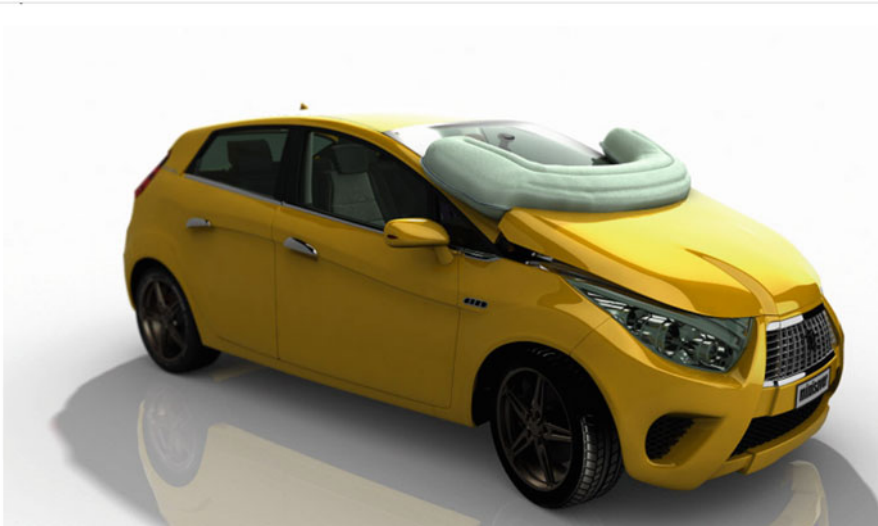
Fig. 4 Example of pedestrian passive safety protection devices ( https://www.autoliv.com/products/passive-safety/pedestrian-protection )
