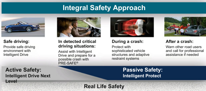
Fig. 1 The Mercedes-Benz concept of “Integral Safety”
