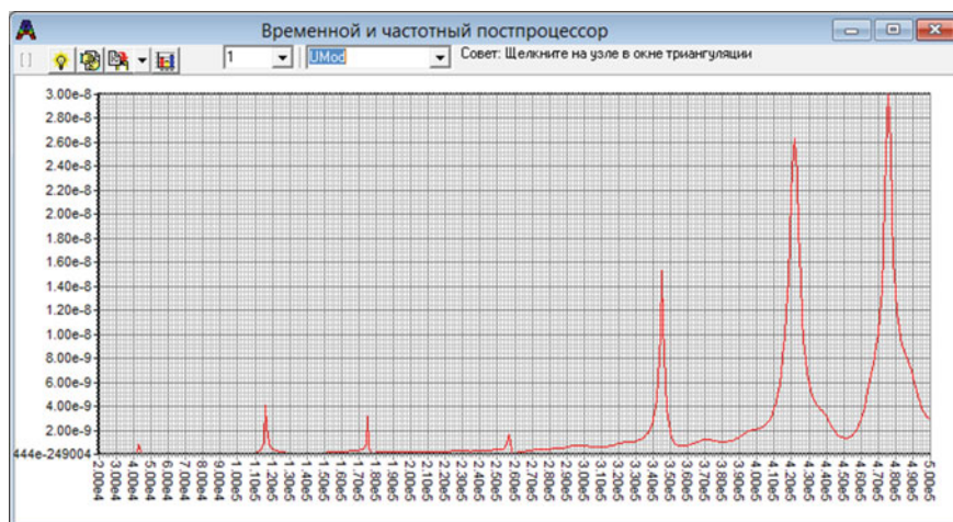
Fig. 21 AFR of the radial displacement
