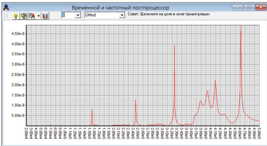
Fig. 13 AFR of axial displacement
