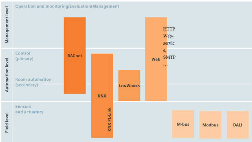
Fig. 24 Communication protocols can cover different level of BMS. (Source Siemens Building Technologies [31])
