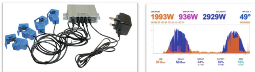
Fig. 52 Open Energy Monitor device with four current measurement, and monitoring
