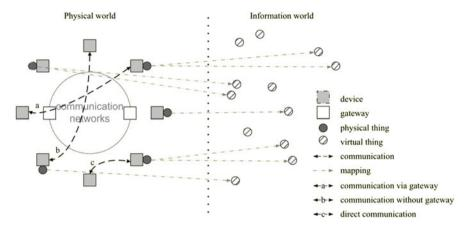
Fig. 29 Technical overview of the IoT and interactions between physical devices [39]
