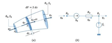
Fig. 3 Steady-state thermal conduction: (a) stream tube; (b) thermal network model
