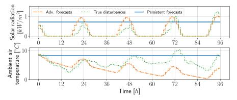
Fig. 18 The persistent forecasts against the advanced disturbance forecasts. The latter is computed by integrating (63) forward using the current observations as initial conditions
