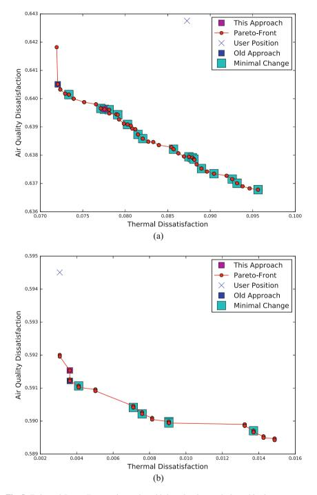
Fig. 5 Estimated Pareto-Fronts using real-world data showing equivalent objective vectors are distributed over the entire Pareto-optimal surface where cyan square objective vectors correspond to action schedules having equal deviation from the historical schedule, blue square and violet
