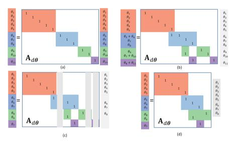
Fig. 10 Obtain matrix temperature nodes  $A_{d\theta}$ : (a) create diagonal matrix; (b) add the column of the second node to the column of the first node in merging:  $[1 5 2 1] \rightarrow \text{col5} = \text{col5} + \text{col6}$ ;  $[2 2 3 2] \rightarrow \text{col7} = \text{col7} + \text{col10}$ ;  $[2 3 4 1] \rightarrow \text{col8} = \text{col}$ . 8 = col11; (c) delete the columns of the second node in merging; (d) obtain matrix  $A_{d\theta}$
