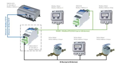
Fig. 25 Automatic meter reading using Filed bus (M-Bus & Modbus) connected to the automation level using Ethernet physical support and TCP/IP protocols. (Source: http://energycare.dk/ portfolio-item/meter-gateway/)
