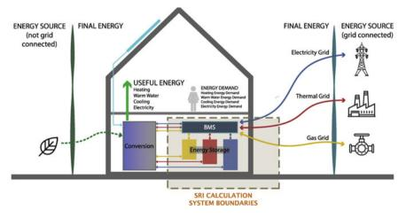
Fig. 12 System boundaries of SRI calculation. (Source: Verbeke et al. [19])
