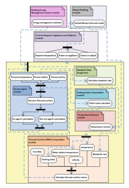
Fig. 26 Co-simulation between inhabitant's behaviour, SIMBAD and BEMS
