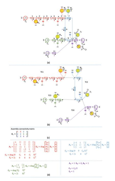
Fig. 5 Example of the problem of assembling thermal circuits: given four circuits, assemble them knowing the common nodes. (a) Assembled circuit. (b) Four disassembled circuits. (c) Assembling matrix. (d) Algebraic description of each disassembled circuit
