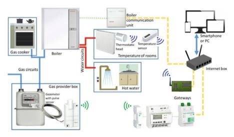
Fig. 39 Typical IoT for gas-based heating and hot water consumption monitoring
