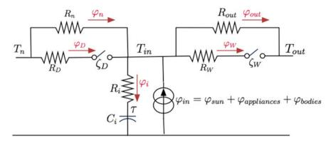
Fig. 8 Lumped element model for the H358 office
