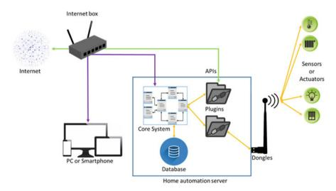
Fig. 46 Smart Home solution with local server implement of low-cost nano-computer
