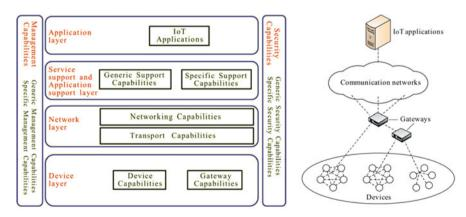
Fig. 32 Four level layers of IoT reference model [39]
