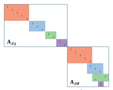
**Fig. 12** Block matrix for  $\begin{bmatrix} \boldsymbol{q}_1^T & \boldsymbol{q}_2^T & \boldsymbol{q}_3^T & \boldsymbol{q}_4^T & \boldsymbol{\theta}_1^T & \boldsymbol{\theta}_2^T & \boldsymbol{\theta}_3^T & \boldsymbol{\theta}_4^T \end{bmatrix}^T$  (first flow branches, then temperature nodes)
