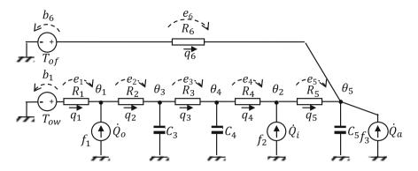
Fig. 16 Temperature nodes are ordered so that the capacity matrix contains zero-blocks
