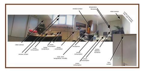
Fig. 14 Office with sensors: the only possible actions are window and door openings during summer
