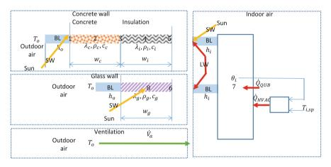
Fig. 7 Model for components to be assembled
