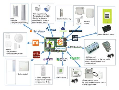
Fig. 54 G2Elab Smarthouse devices and multi-protocol gateway
