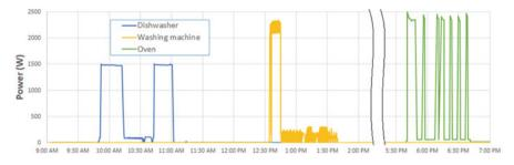
Fig. 53 Three main power consumption profiles of home electric appliances
