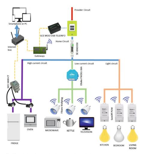
Fig. 37 Typical IoT for home electrical consumption monitoring
