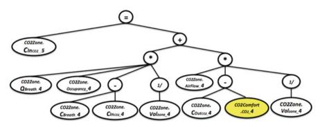
Fig. 10 CO<sub>2</sub> zone model after the ODE transformation process
