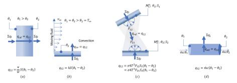
Fig. 2 Conductances in heat transfer and energy advection: (a) conduction; (b) convection; (c) radiation; (d) advection
