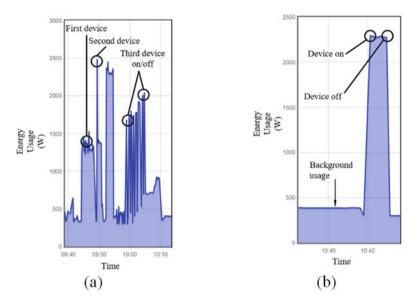
Fig. 4 Aggregated load readings highlighting unique device signatures
