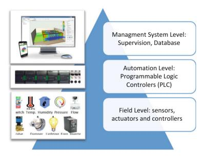
Fig. 21 Architecture of a building automation and control system
