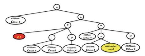
Fig. 11 CO<sub>2</sub> zone binary model after the first linearization process
