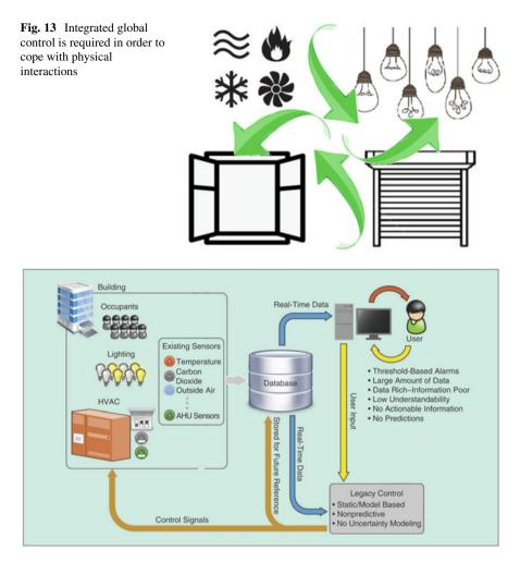
Fig. 14 Typical building automation system. (Source: Manic [23])
