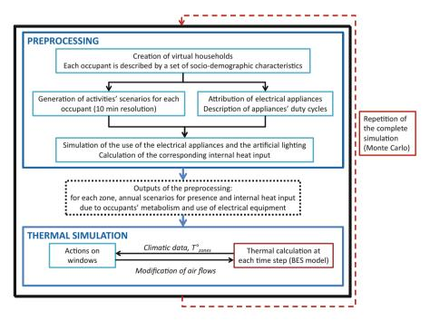
Fig. 33 Algorithm of the integrated behavioural model coupled to the DBES tool
