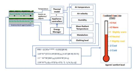
Fig. 27 Fanger's model in co-simulation
