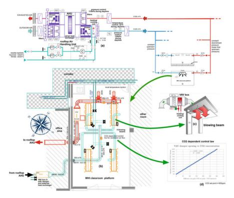
Fig. 2 MHI classroom platform and its HVAC system
