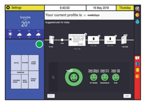
Fig. 17 At-one-click human control and recommendations. The action plan consists of a sequence of actions recommended to users in order to maintain comfort in conformity with their preferences
