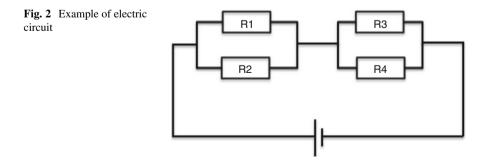
such a pivot model can be done by composing first a bloc of 2 parallel resistors. Then, the pivot model is built by duplicating this bloc and connecting the whole system.
