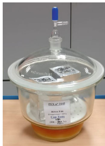
(a) Schematic illustration of the glass cup (b) Setup with the desiccator setup
