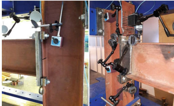
Fig. 8 a Beam end plate (of cantilever beam) attached by means of clamps to the pillar. b Cuts made in the pillar flange to research the profile effective length by means of the tests
