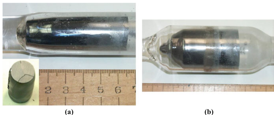
Fig. 6 The pictures of two as-grown CdZnTe ampoules. (a) CZT-39 ampoule: without HF treatment resulted in the sample separating axially into three pieces as shown by the inset; (b) CZT-36 ampoule: with HF treatment, as-grown sample detached and slid inside the ampoule
