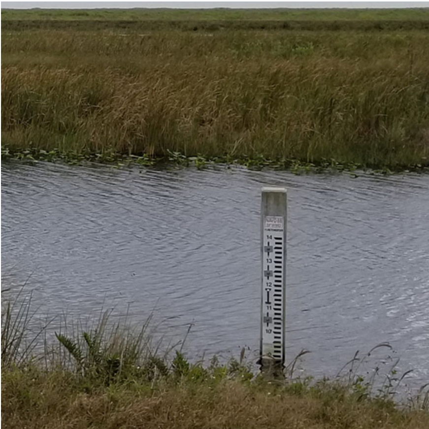
Fig. 16.3 Staff gauge for reading stage or water level (Photo by Wossenu Abteu)
