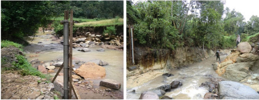
Fig. 26.6 Crest stage gauge installation at station 2 (left photo) and station 6
