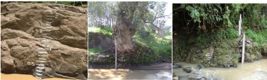
Fig. 26.5 Examples of staff levels, painted on natural rock, metal meter section mounted on eucalyptus poles and modern staff gauge
