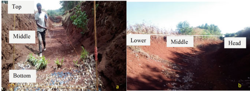
Fig. 21.3 Soil sampling locations within the investigated gullies, soil sampling along the gully depth for bulk density analysis (a) and soil sampling along the gully length for soil texture analysis (b)
