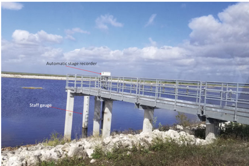
Fig. 16.4 Manual and automatic stage recorders (Photo by Wossenu Abteu)
