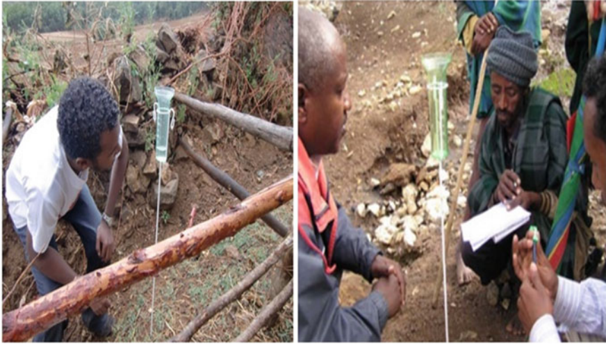
Fig. 26.3 Simple garden rain gauges were used at the MMP stations
