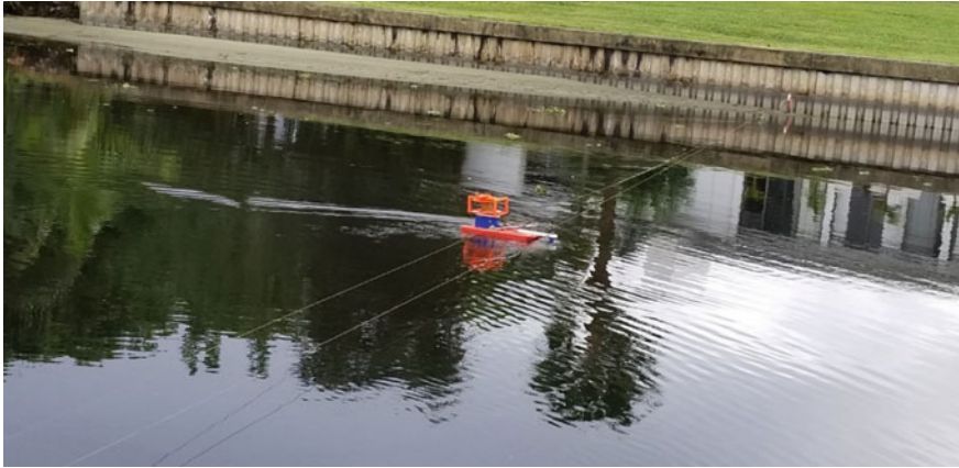
Fig. 16.2 StreamPro ADCP measuring flow across a canal (SFEC 2020)
