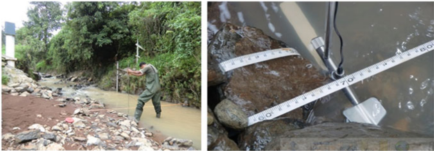
Fig. 26.4 Current meter measurement with current meter at station 11
