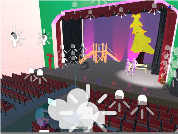
Fig. 1. The Keylight stage with a lighting design. The icons show where lights are hung in the space, with different types for the house and stage lights. A large camera icon intersects with a table light near the bottom of the image. This shows where the user sits in virtual reality, next to the board operator at a table in the house.
