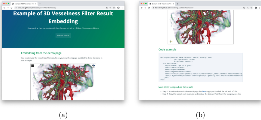
Fig. 7. Example of 3D result embedding in other web pages. (a) Interactive 3D viewer embedded in a GitHub web page. (b) HTML container source code with main steps to construct the given page.
