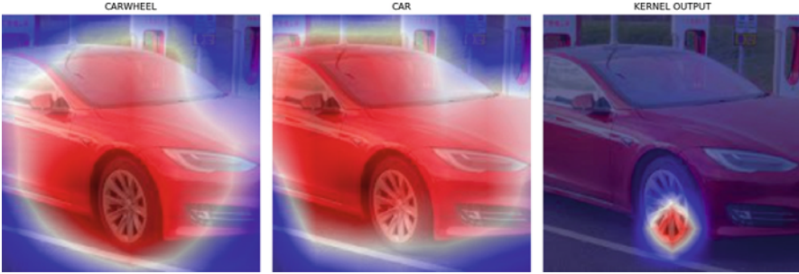
Fig. 7.6 Example of Amplified Directed Divergence kernel applied to class activation maps computed from two expert models. The first image shows the class activation map computed on a car wheel classification from an expert model trained to classify car wheels. The second image shows a class activation map on a car classification from an expert model for cars. The third image shows a class activation map that better localizes the target class (car wheel) computed using the kernel method
