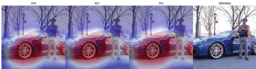
Fig. 7.5 The same input image as in Fig. 7.4 and Class Activation Maps are computed for three ImageNet classes of interest, car wheel, race car, and sports car. This method is not prone to result in attention on spurious features. However, as can be seen from the three leftmost images, significant overlap exists between the classes for which CAMs were computed
