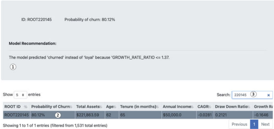
Fig. 4.9 Model Recommendation screen. ① The verbalization explanation contrasting the fact and the foil. ② The table allows users to change the explanation to another instance and also visualize the feature values for the instances. ③ The search function enables users to search for specific instances
