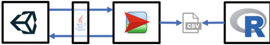
Fig. 4.1 High-level system diagram for all ASSOC modules and their connections. Unity and NetLogo communicate through a Java relay app. NetLogo writes simulation output to a csv file, which is the input for R
