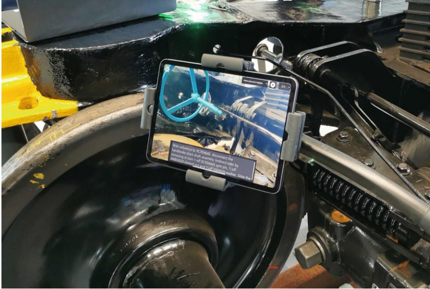
Fig. 8.9 Example of an AR overlay for identifying service and maintenance items on a train chassis
