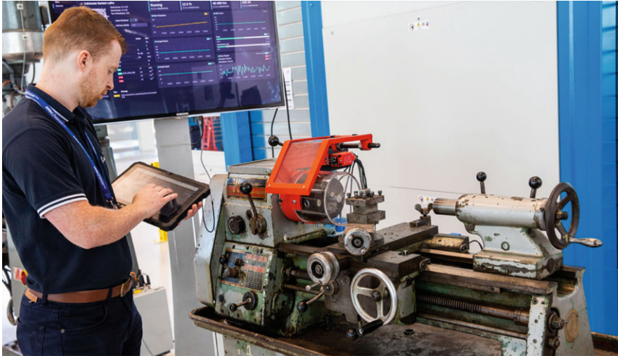
Fig. 8.4 Colchester Bantam lathe with a low-cost Industry 4.0 solution (Lockwood et al., 2018)
