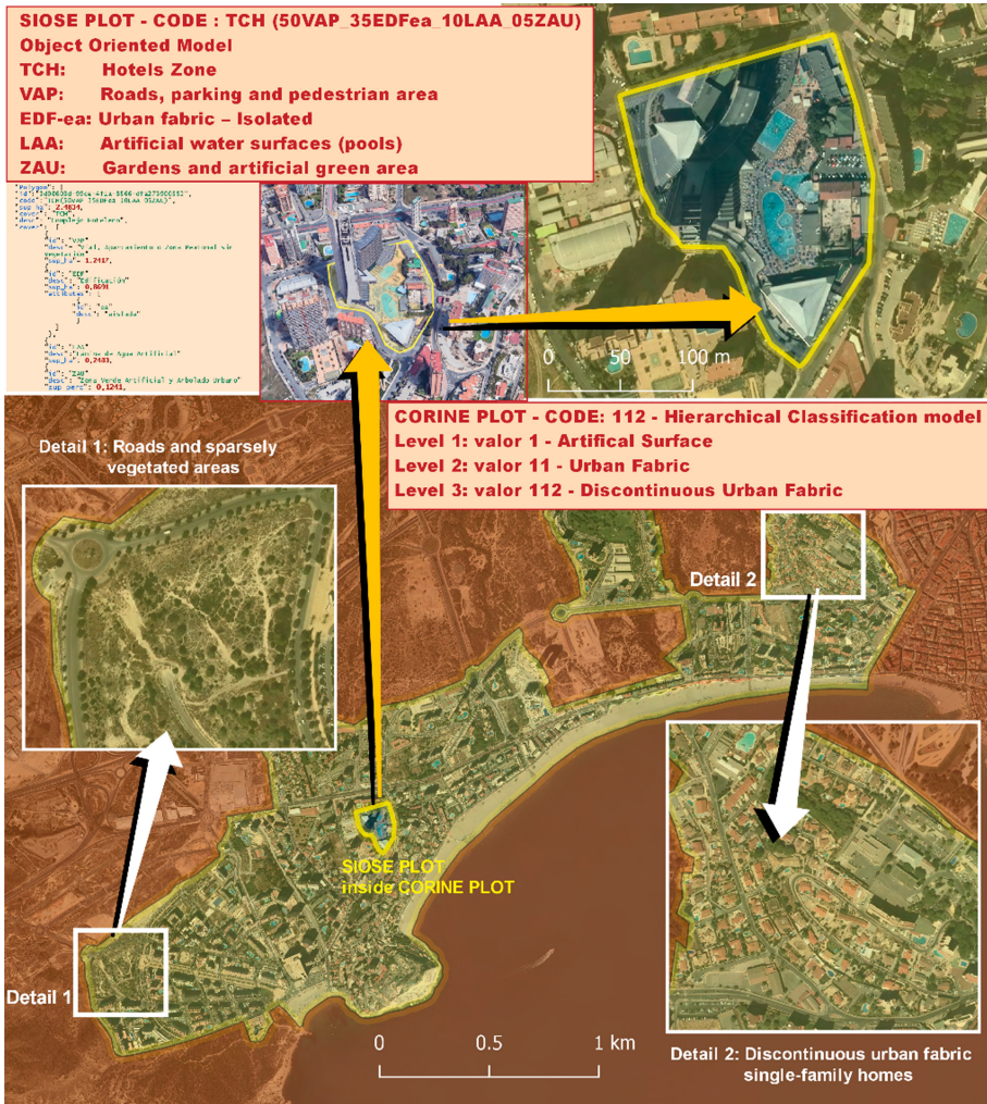
Fig. 2. Detail of same area of Benidorm (SE of Spain). Example of the treatment of the thematic LULC information between Corine LC hierarchical model and SIOSE object-oriented model. Source: Corine LC, SIOSE and aerial orthophotography flight from National Geographic Institute (PNOA) and Google Earth.
