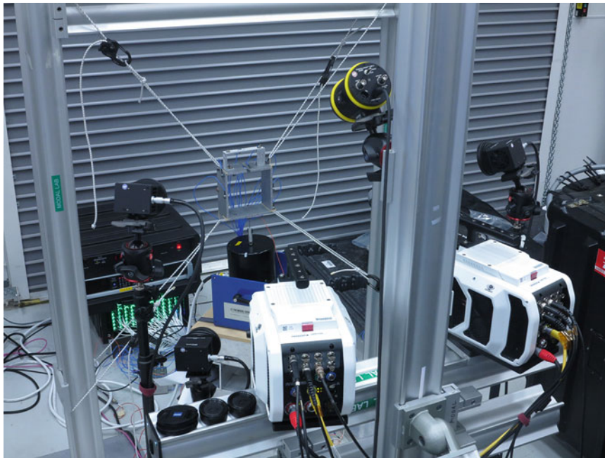
Fig. 3.7 Example stereo DIC test of the BARC structure
