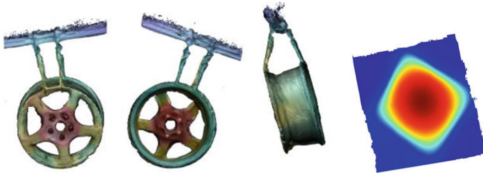
Fig. 1.9 Three different views from the third mode (1215 Hz) of car rim. Seventh mode (528 Hz) of steel plate without texture
