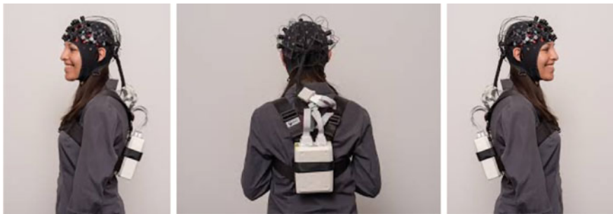
Fig. 2 Example of an ultra-portable fNIRS imager: NIRSport by NIRX Medical Technologies, LLC
