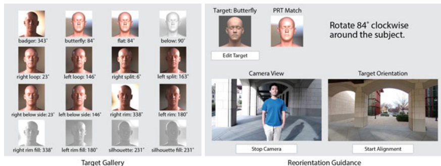
Fig. 2 Upon loading an HDR environment map of the current scene, the interface of our portrait lighting tool computes the optimal orientation for each target lighting style and displays a gallery of target appearances (left). The tool grays out unattainable targets. Selecting a target brings up the reorientation guidance screen, which displays how far the photographer should rotate clockwise or counterclockwise around the subject (right). It also shows the background at the target orientation and the current view from a webcam at the current location of the photographer
