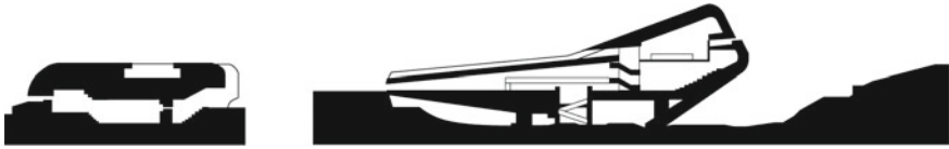
Fig. 1 The figure represents a comparison between a German Bunker structure analyzed by P. Virilio in his collection of drawings between 1958 and 1963 [4] (left) and the project of C. Parent and P. Virilio of the Cultural Centre of Charleville, built in 1966 (right). A. Monacelli's drawing
