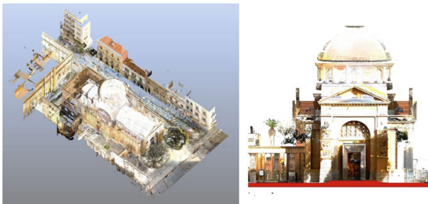
Fig. 9 Church of St. George: axonometric view of the point cloud of the and main façade (graphic elaboration by Francesco De Lorenzo)
