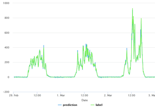
Fig. 11. FMLP-NN for forecast February from 29 to March 02, 2020 using solar radiation and wind speed.
