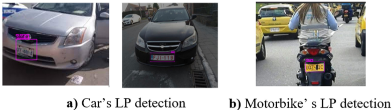
Fig. 4. Results of our LP detection system for (a) Car and (b) Motorbike
