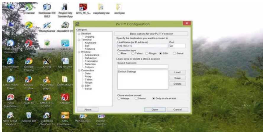
Fig. 4.7 (a) PuTTY which enables user to connect Pi server. (b) PuTTY configuration enabling the SSH of X1 forwarding
