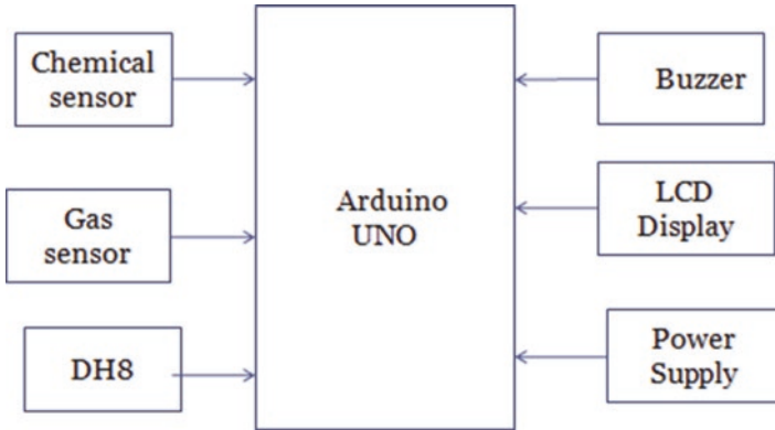
Fig. 3.11 Sewage alert monitoring system
