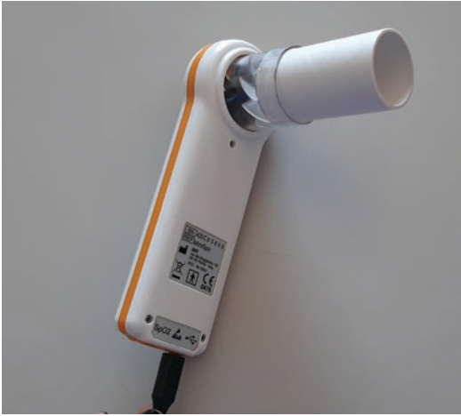
Fig. 28.1 Turbine flow meter spirometer
