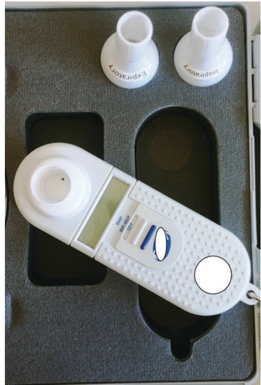
Fig. 3.1 A portable machine for the measurement of maximal inspiratory and expiratory pressures
