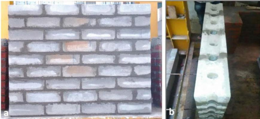
Fig. 17.32 Stretcher bonded hollow block wallette kept for curing: a front view, b top view
