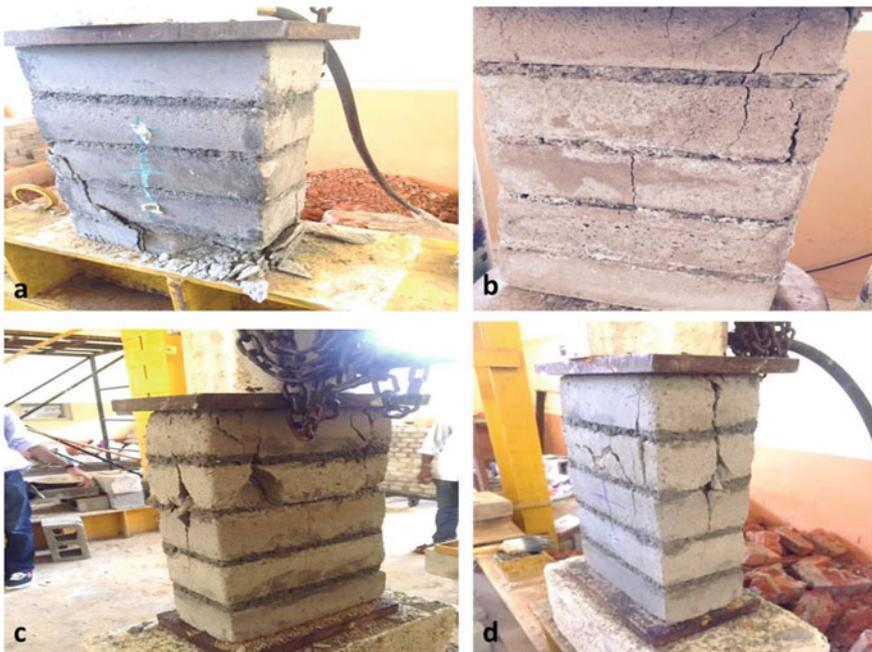
Fig. 17.15 Failure pattern of brick prisms
