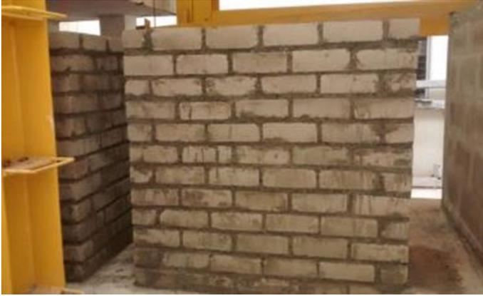
**Fig. 17.24** Stretcher bonded geopolymer brick wallette kept for curing
