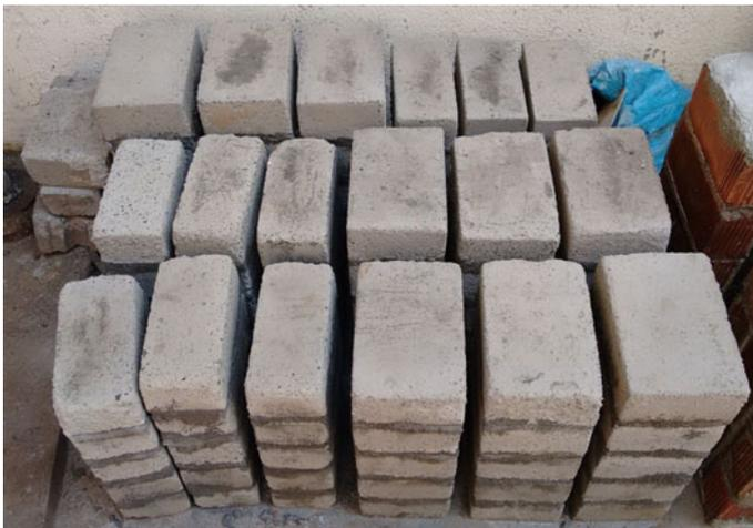
**Fig. 17.10** Stack bonded prisms
