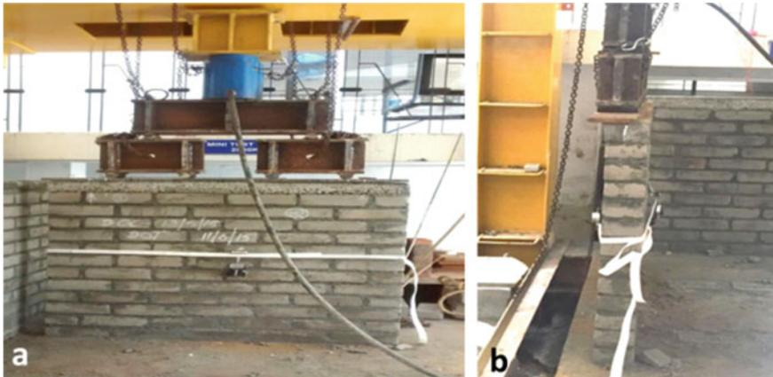
**Fig. 17.25** Ladder arrangement for geopolymer brick wallette: **a** axial loaded brick wallette, **b** eccentric loaded
