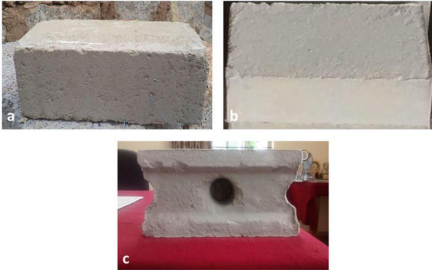
**Fig. 17.3** a Geopolymer bricks, b geopolymer solid block, c geopolymer hollow block
