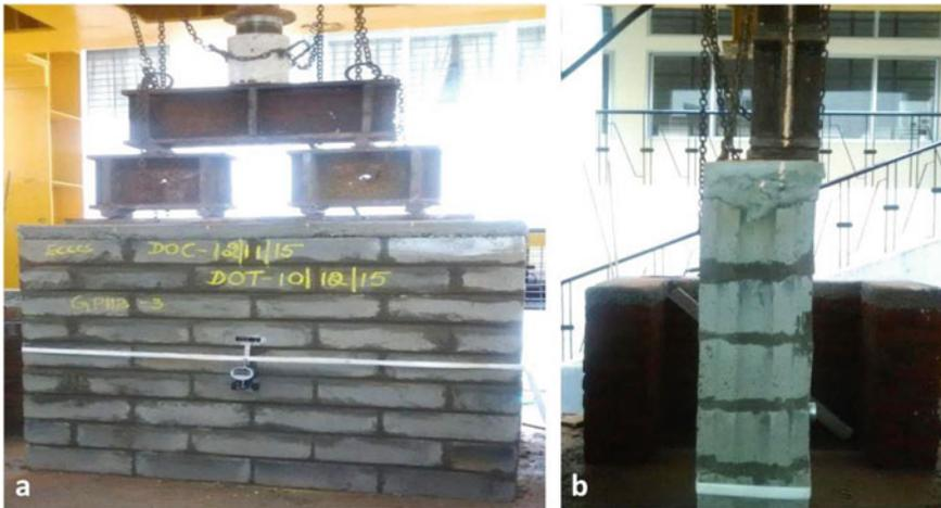
**Fig. 17.33** Ladder arrangement for geopolymer hollow block wallette testing: **a** axial loaded wallette, **b** eccentric loaded
