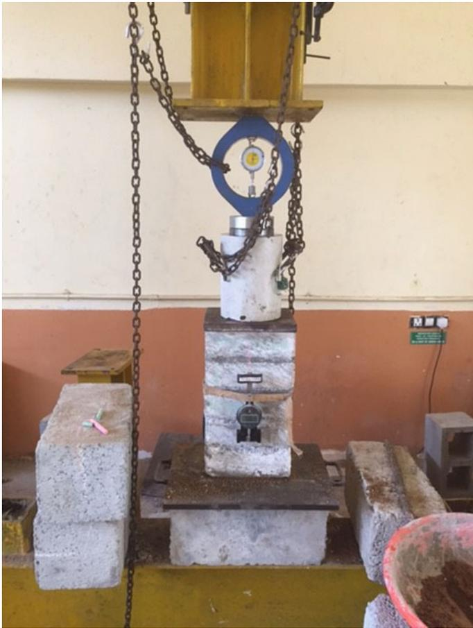
**Fig. 17.19** Testing arrangement of geopolymer hollow block stack bonded prisms
