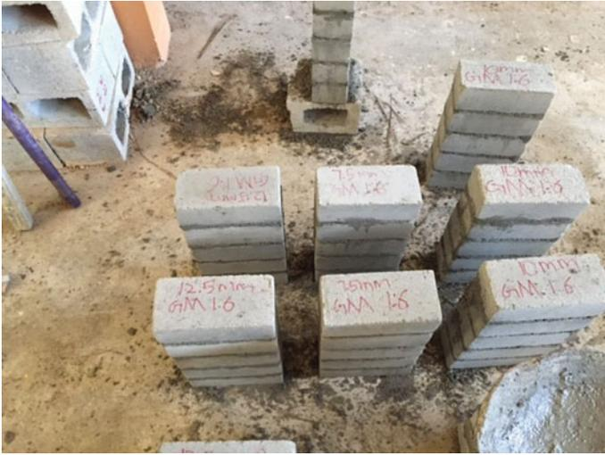
**Fig. 17.11** Unrendered stack bonded prisms
