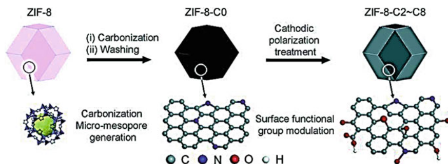
Fig. 4 Carbonization of ZIF-8 results in forming a highly porous template (Reproduced with permission from [86].)
