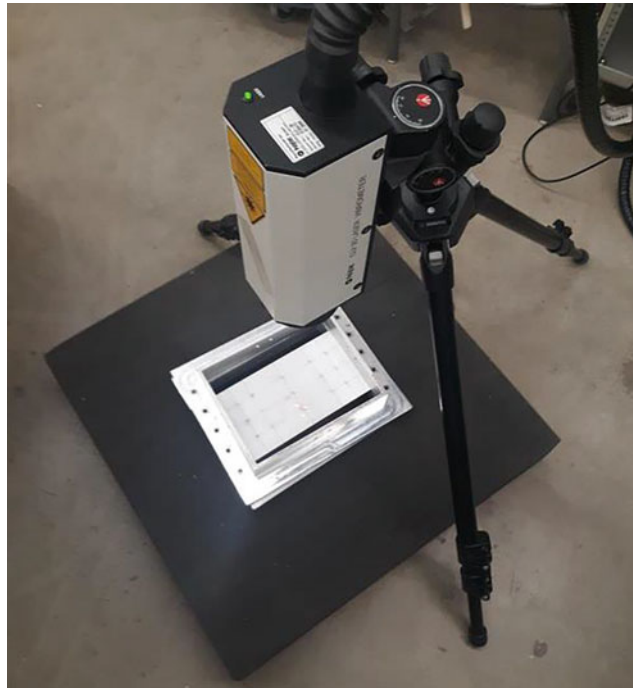
Fig. 11.2 Impact testing setup showing vibrometer and foam holder with test fixture
