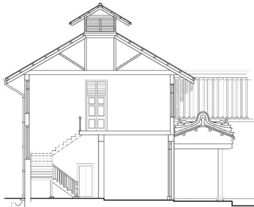
Fig. 10. Section of the newly-altered two-story dormitory in 1906 showing the use of a Western roof truss system. Personal collection.
