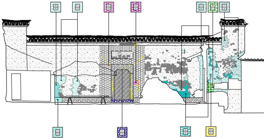
Fig. 9. Complete drawing with the various pathologies in a facade, including the indication symbols for each pathology.
