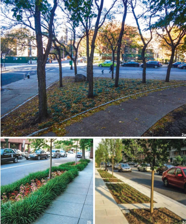
Fig. 27.2 Examples of open soil volume tree planting beds. (a) cluster planting Ft. Greene, Brooklyn NY (Credit C. Glaeser); (b, c) extended curbside tree planting beds with pedestrian access. (Credit: Casey Trees, Washington D.C.)
