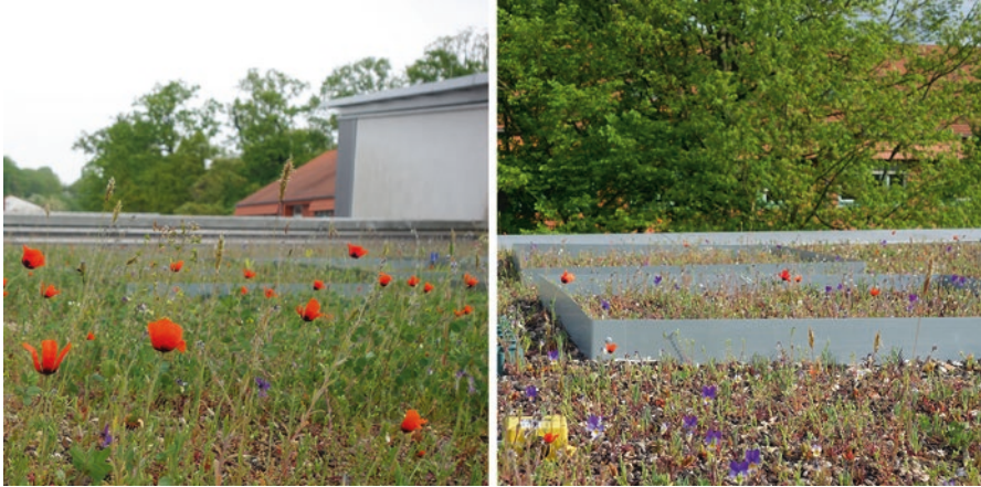
Fig. 6.2 Green-roof experiments started in late summer 2018 testing the establishment of native dry grassland species on EGR types I (left) and III (right) at the library and lecture building of Osnabrück University of Applied Sciences (for details, see Table 6.3). Flowering aspect of annual species (e.g. Viola tricolor , Papaver argemone ) in May 2019, eight months after sowing. (Photo credit: Daniel Jeschke)
