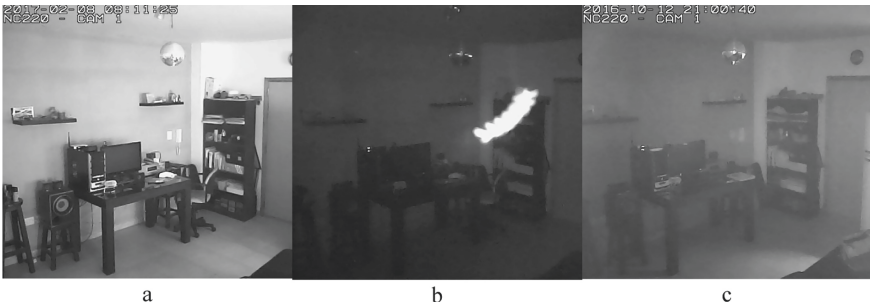
Fig. 2. Examples of false positives informed by the background subtraction based motion detector of the camera: a) during daylight; b) at night, generated by brightness reflected on any of the objects in the image; c) at night (Source: own)
