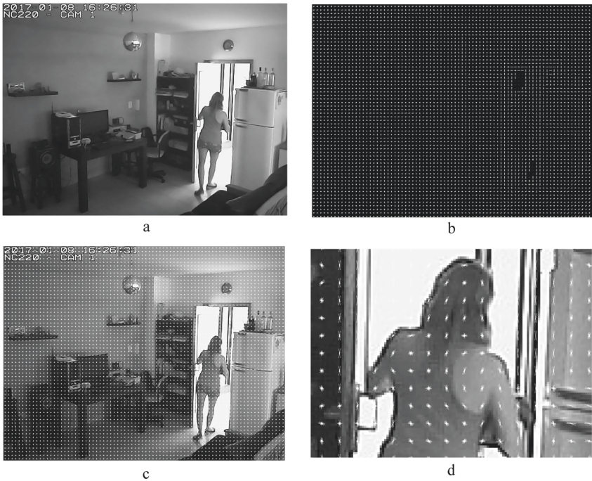
Fig. 3. Visualization of the descriptors of histograms of oriented gradients in images with people a) Original image b) Oriented gradients of the original image c) Superposition of the gradients on the original image d) Detail of the orientation of the gradients in the area where a person is viewed (Source: own)
