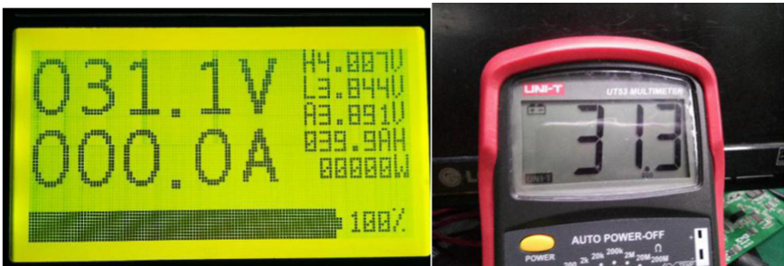
Fig. 10. Comparison of the voltage detected by the system and the measured value
