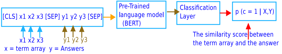
Fig. 4. BERT Fine Tuning: The term array X and the candidate answer Y are combined to form an input to the BERT model (pre-trained) for fine-tuning.
