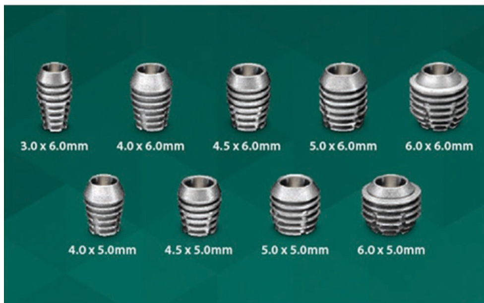
Fig. 15.4 Implant design features of Bicon Short® Implants (Bicon Corp., Boston, MA) include a wide-diameter threaded design with a locking taper that has an inherent platform switch mechanism. (Reproduction with permission from Bicon Dental Implants)
