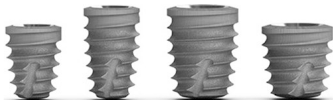
Fig. 15.5 Implant design features of BioHorizons Tapered Short® Implant (BioHorizons, Birmingham, AL) include an aggressive thread profile, platform switching features, and an implant collar with laser-ablated dual-affinity microgrooves (Laser-Lok®) for crestal bone retention and connective tissue attachment. (Reproduction with permission from BioHorizons)
