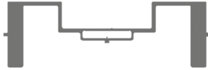
Fig. 1. Inlay under development used S_{11} and realized gain measurements.
