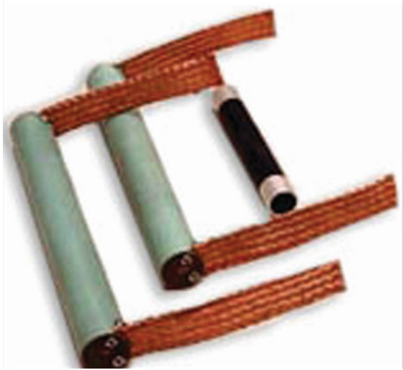
Fig. 3.13 Bulk and encased current leads marketed by M/S 'Can Superconductors' and used in author's lab (IUAC New Delhi)
