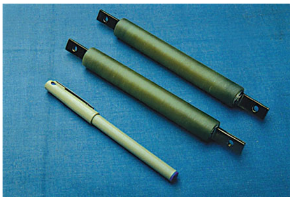
Fig. 3.14 Pair of 100 A, BSCCO-2223 current leads developed by NIIST, Thiruvananthapuram. Leads with higher current rating available [8]. Courtesy R. P. Aloysius
